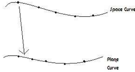
Figure 7. Projection problem for curves vs. projection problems for lists of points.
